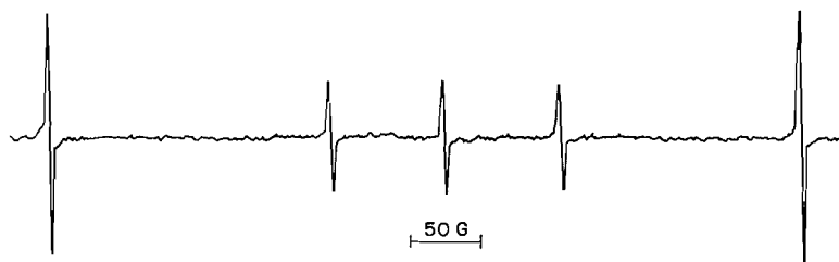
FIG. 6. "Low-power" EPR spectrum of tritiated \text{HClO}_4 + \text{H}_2\text{O} + \text{D}_2\text{O} mixture at liquid nitrogen temperature. The spectrum consists of two H and three D lines.
